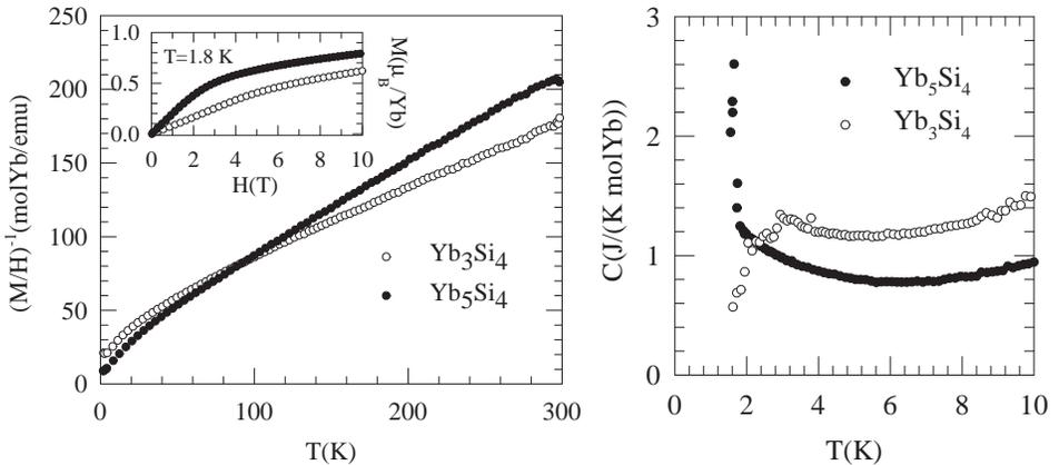
Fig. 1. Left: inverse magnetic susceptibility in  $\text{Yb}_5\text{Si}_4$  and  $\text{Yb}_3\text{Si}_4$ ; inset: magnetisation curves at 1.8 K. Right: Heat capacity in  $\text{Yb}_5\text{Si}_4$  and  $\text{Yb}_3\text{Si}_4$ .
