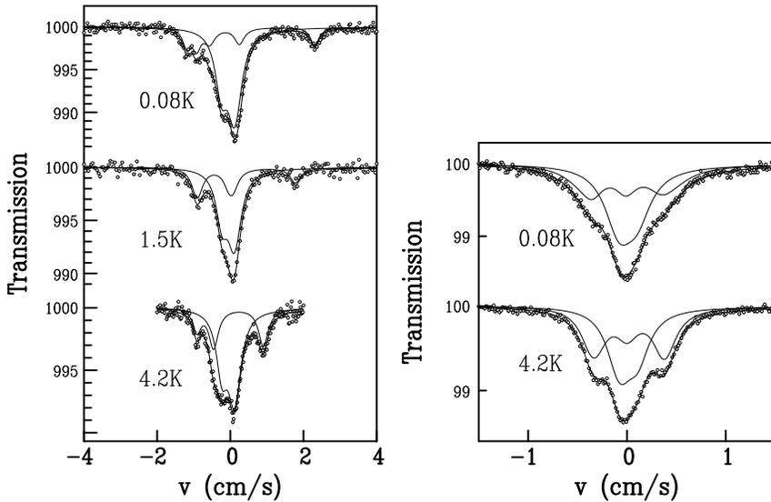
Fig. 2. Left:  $^{170}\text{Yb}$  Mössbauer spectra in  $Yb_5Si_4$  at 80 mK, 1.5 and 4.2 K. The subspectrum with the largest splitting corresponds to  $\text{Yb}^{3+}$  with magnetic ordering. Right:  $^{170}\text{Yb}$  Mössbauer spectra in  $Yb_3Si_4$  at 80 mK and 4.2 K. The two subspectra have equal intensities, and that with the largest splitting shows a line-broadening at 80 mK which could indicate magnetic ordering of  $\text{Yb}^{3+}$  ions.
