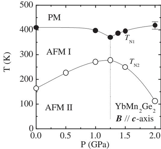
Fig. 2.  $P$ - $T$  phase diagram of  $\text{YbMn}_2\text{Ge}_2$ . Where, the solid and open circles represent  $T_{N1}$  and  $T_{N2}$ , respectively, and the value of  $T_{N1}$  under  $P = 2.0$  GPa was estimated from the values of  $T_{N1}$  below 1.5 GPa. Broken line represents a critical pressure at which an occurrence of magnetic structural change is expected.
