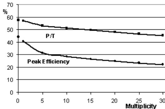
Fig. 4. Efficiency and  $P/T$  of AGATA as a function of multiplicity for cascades of 1 MeV  $\gamma$ -transitions. The values are based on a tracking efficiency of about 50% which is likely to be improved in the near future.
