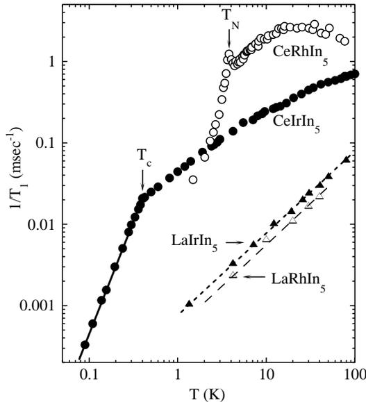
Fig. 1.  $T$ -dependence of  $^{115}(1/T_1)$  for  $\text{Ce}(\text{Ir,Rh})\text{In}_5$  and the reference compounds  $\text{La}(\text{Ir,Rh})\text{In}_5$ . The solid and dashed lines indicate the  $1/T_1 \propto T^3$  and  $1/T_1 \propto T$  relations, respectively.
