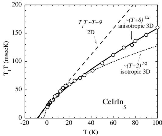
Fig. 2.  $T_1 T$  plotted as a function of  $T$  for  $\text{CeIrIn}_5$  above  $T_c$ . The broken line, solid and dotted curves are the  $T$ -variations of  $T_1 T \propto T + \theta$  (2D SFs),  $T_1 T \propto (T + \theta)^{3/4}$  (anisotropic SFs) and  $T_1 T \propto (T + \theta)^{1/2}$  (3D SFs), respectively.
