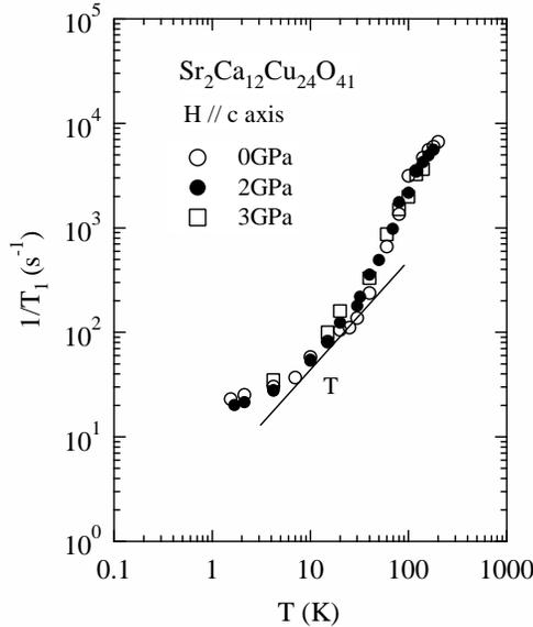
Fig. 1.  $1/T_1$  of  $^{63}\text{Cu}$  nuclei on ladder sites.
