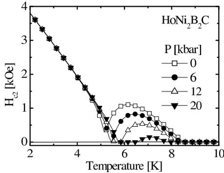
Fig. 2. Theoretical calculations have been made using the model given in Ref. [3] of the temperature dependence of  $H_{c2}$  for  $\text{HoNi}_2\text{B}_2\text{C}$  for several pressures (see the text).
