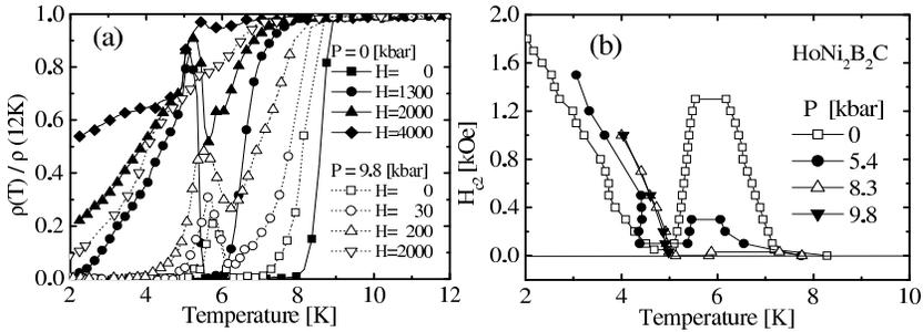
Fig. 1. Temperature dependence of the resistivity of  $\text{HoNi}_2\text{B}_2\text{C}$  for several magnetic fields at ambient pressure (closed symbols) and 9.8 kbar (open symbols). Temperature dependence of  $H_{c2}$  for several pressures.
