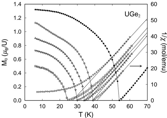
Fig. 2. Temperature dependence of the spontaneous magnetization  $M_0$  and inverse susceptibility  $1/\chi$  which were obtained from the Arrot plot. The symbols are as follows:  $P = 0$  kbar ( $\bullet$ ), 9.1 kbar ( $\circ$ ), 12.3 kbar ( $\triangle$ ), 12.9 kbar ( $\nabla$ ), 15.0 kbar ( $\square$ ) and 16.9 kbar ( $\diamond$ ).
