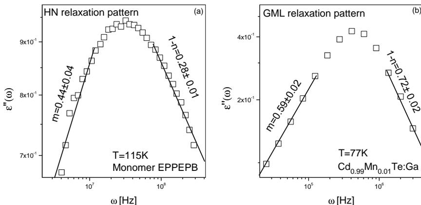
Fig. 2. Various non-exponential relaxation patterns in real systems. The HN dielectric response (a) was observed by Włodarska *et al.*, in liquid crystalline epoxy monomer EPPEPB [7]. The GML relaxation (b) was observed by us in gallium (Ga) doped semiconducting mixed crystal  $\text{Cd}_{1-x}\text{Mn}_x\text{Te}$  of  $x = 0.01$  manganese (Mn) content.
