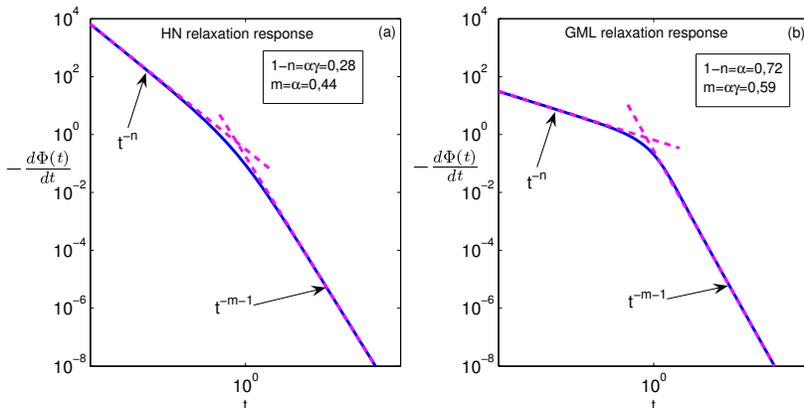
Fig. 3. Sample time-domain representation of the Havriliak–Negami and the generalized Mittag–Leffler responses. Values of the power-law exponents as for the experimental data presented in Fig. 2.
