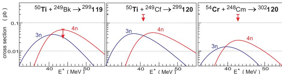
Fig. 2. Predicted cross sections for the production of new elements 119 and 120 in the Ti and Cr induced fusion reactions [9]. The arrows indicate the upper limits reached in the corresponding experiments performed at GSI [10, 11].
