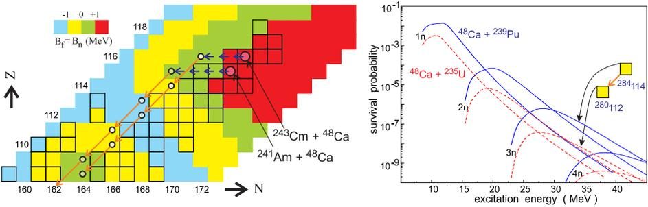
Fig. 3. The values of  $B_f - B_n$  as a function of proton and neutron numbers. Known isotopes of SH elements are marked by the bordered rectangles. The right panel shows the survival probability of CN  $^{283}112$  and  $^{287}114$  formed in the fusion reactions  $^{48}\text{Ca} + ^{235}\text{U}$  (dashed curves) and  $^{48}\text{Ca} + ^{239}\text{Pu}$  (solid curves).
