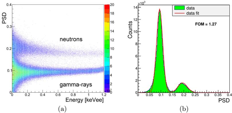
Fig. 6. (a) An example of neutron- $\gamma$  discrimination plot obtained with a stilbene scintillator under irradiation of  $^{252}\text{Cf}$  source; (b) FOM value for the lower energy threshold  $\sim 75$  keVee. Data fit is performed by a default ROOT build in procedure using a Gaussian function.
