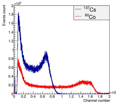
Fig. 5. The scintillation amplitude spectra for the stilbene crystal irradiated by  $\gamma$  rays from  $^{137}\text{Cs}$  and  $^{60}\text{Co}$  sources.
