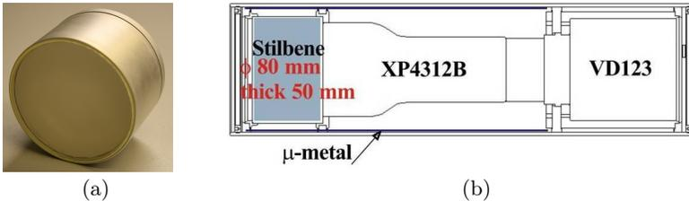
Fig. 2. (a) Stilbene scintillator of 80 mm in diameter and 50 mm thick encapsulated into an aluminum housing. (b) A scheme of a detection module.
