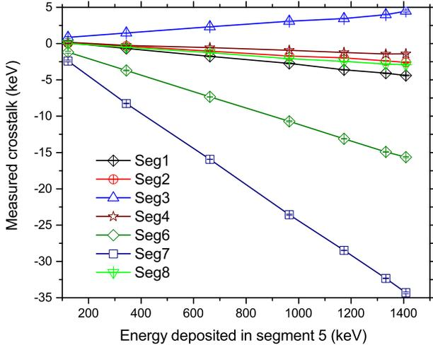
Fig. 2. Measured crosstalk on the non-hit segments of crystal A when segment 5 in crystal A was hit. The crosstalk energy is a linear function of the energy deposited in segment 5.
