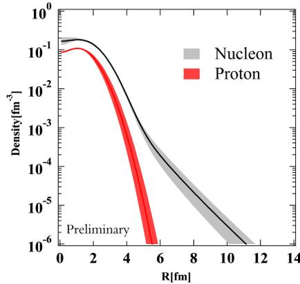
Fig. 4. (Color online) Density distributions of  $^{16}\text{C}$ : Nucleon density distribution (lighter/gray line) deduced from  $\sigma_R$  on nuclear targets, where shade area represents the error. Darker/red line and shade area represent proton density distribution and its error, deduced from  $\sigma_R$  on proton targets. The difference between them is the neutron density.
