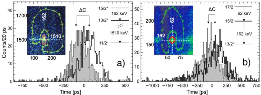
Fig. 2. Time spectra employed in the lifetime analysis of the  $13/2^+$  (left) and  $15/2^+$  (right) states. Dark (light) histograms are the delayed (anti-delayed) time difference for the cascades shown in the right part of each picture. Examples of two-dimensional background selections are given in the insets.
