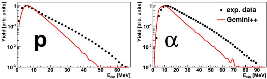
Fig. 2. Energy spectra of protons and  $\alpha$  particles emitted between  $7^\circ$  and  $17^\circ$  in the F-E channel of the reaction  $^{32}\text{S}+^{48}\text{Ca}$  at 17.7 MeV/u (experiment “III”).
