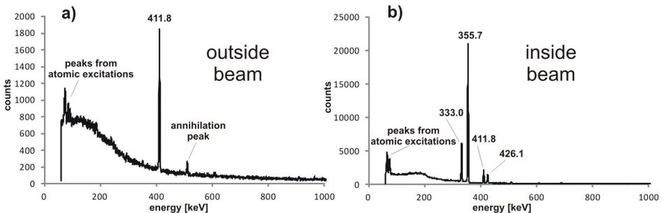
Fig. 1. Spectra of the produced radioisotopes of gold.
