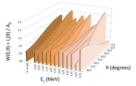
Fig. 2. Pseudo-3D plot of the fit results to the measured angular distributions of prompt  $\gamma$  rays from <sup>252</sup>Cf(sf) according to Eq. (1). Shown is the angular distribution obtained for the entire energy spectrum to the left together with those for the individual energy bins. Please, observe that for the latter, the axis description gives the center of each bin.
