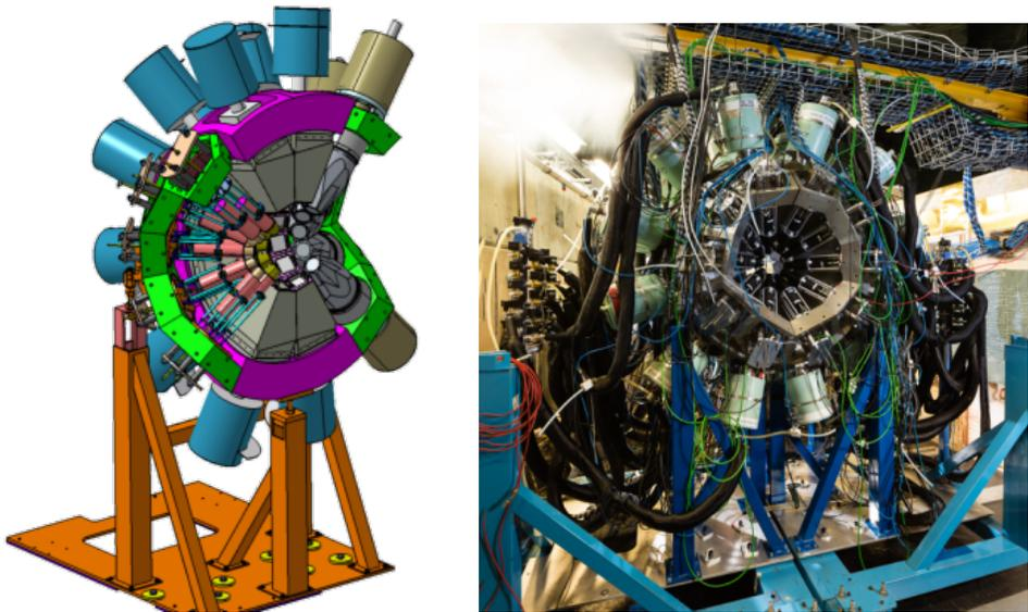
Fig. 1. (Colour on-line) Left — CAD drawing of half of the  $\nu$ -ball array. LaBr<sub>3</sub> detectors are black/pink. On their right, the BGO shields of the clover detectors are drawn. Phase I HPGe detectors are symmetric to LaBr<sub>3</sub>, with respect to clovers. Right — a photo of the  $\nu$ -ball array before the commissioning experiment is presented.
