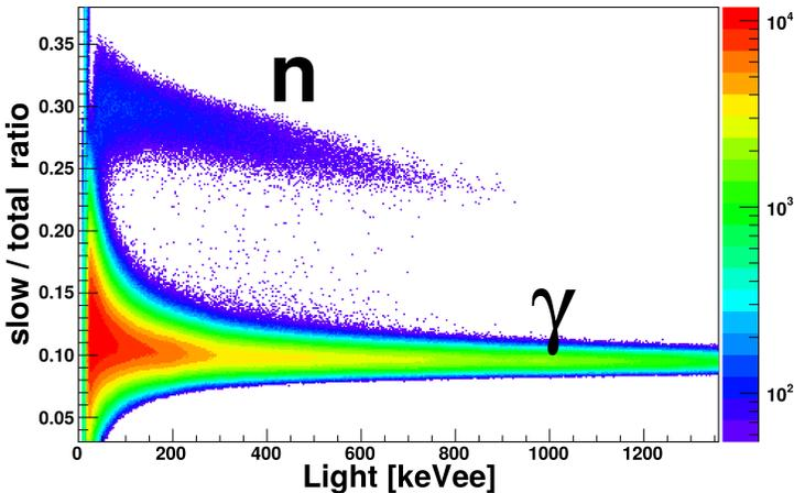
Fig. 1. Neutron-gamma discrimination using the charge comparison method [15]. The spectrum was obtained with a NEDA detector using a  $^{252}\text{Cf}$  source. The ratio of slow-to-fast signal integrals is plotted *versus* the total light.
