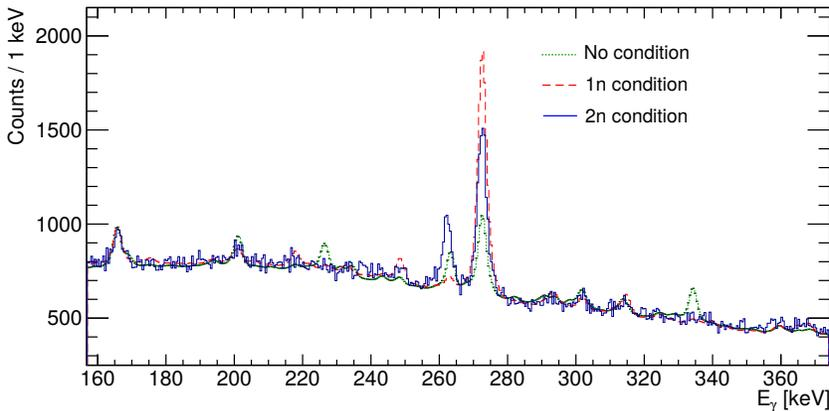
Fig. 3. (Colour on-line) Gamma spectra measured with AGATA spectrometer with a 115 MeV  $^{36}\text{Ar}$  beam and  $^{16}\text{O}$  target, without any condition (dotted green line) and gated on one and two neutrons (dashed red and solid blue lines, respectively) detected in the NEDA array. The spectra are scaled so the background level for all three of them is the same. The Y-axis scale is true for  $1n$  gated spectrum. See discussion in the text.
