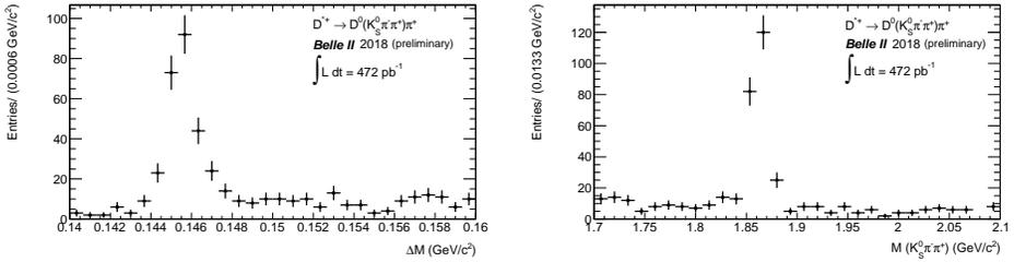
Fig. 2. Distributions of the difference in the invariant masses of  $D^*$  and  $D$  mesons denoted as  $\Delta M$  (left) and the invariant mass of  $D$  meson denoted as  $M_D$  (right) for  $D^{*\pm} \rightarrow D(K_S^0 \pi^+ \pi^-) \pi_{\text{slow}}^\pm$  decays.
