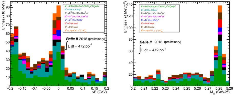
Fig. 3. Distributions of energy difference  $\Delta E$  (left) and beam-constrained mass  $M_{\text{bc}}$  (right) for various  $B$  decay modes with phase II Belle II data.
