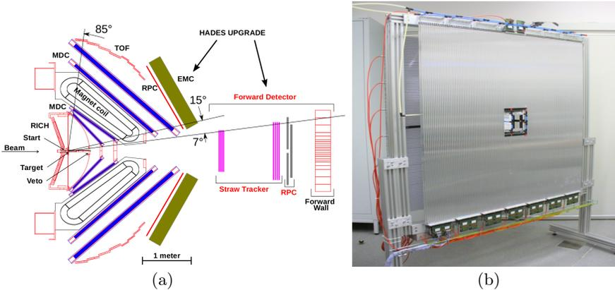
Fig. 1. A cross section of the HADES detector (a) with the installed Forward Detector and Electromagnetic calorimeter upgrade. Two out of six segments are shown. Particles cross the detector from the target through the RICH, two planes of MDC modules, the toroidal magnet, again 2 planes of MDC, the TOF wall and both upgraded systems ECAL and FT (b).
