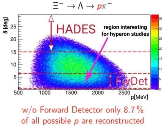
Fig. 3. Observed simulated  $p$  distribution in the forward angles of HADES at 4.5 GeV clearly shows the increase in detection capability.
