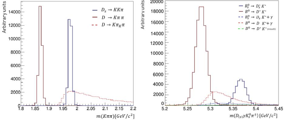
Fig. 2. Left plot: Mass of  $D \rightarrow K\pi\pi$  candidates (grey/red line),  $D_s \rightarrow KK\pi$  candidates (black/blue line) and  $K\pi\pi$  system, where one pion is misidentified as kaon (dashed grey/red, line). Right plot: Mass of  $D_s\gamma K^0\pi$  candidates for signal modes and potential background processes, the dashed histograms show decays combined with the low-energy, random photon (pseudoeperiments produced with RapidSim [4]).
