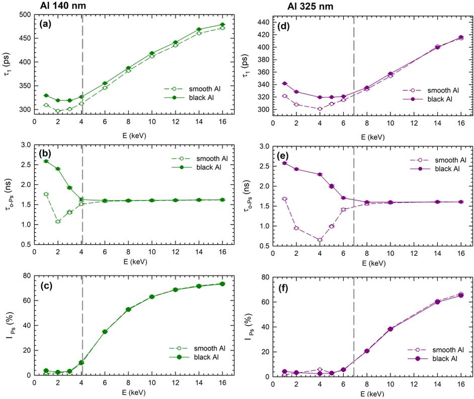
Fig. 2. Results of VEPAS investigations of black and smooth Al films with thickness of 140 nm (a), (b), (c) and 325 nm (d), (e), (f).
