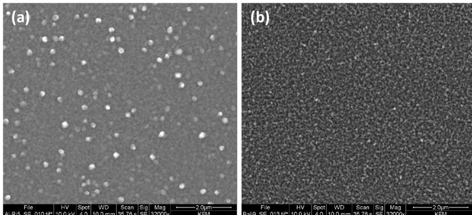
Fig. 1. Secondary electron SEM images of surface of (a) smooth Al film; (b) black Al film with thickness of 325 nm.
