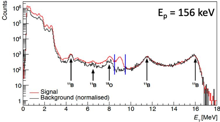
Fig. 2. (Color online) The experimental spectrum for the 156 keV resonance acquired using neon (argon) gas in gray/red (black). The two spectra are normalized to match the region  $E_\gamma = 10.5\text{--}17.0$  MeV. The main sources of beam-induced background are also labeled in the figure.
