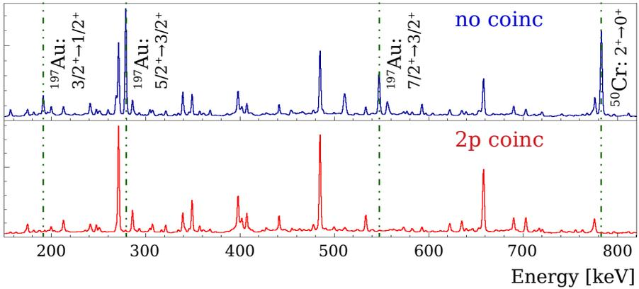
Fig. 1. Comparison between the spectra in coincidence with two protons (bottom) and the total  $\gamma$ -ray spectrum (top) detected at  $152^\circ$  with a target–stopper distance of 10  $\mu\text{m}$ . The suppression of the  $^{50}\text{Cr}$  and  $^{197}\text{Au}$  Coulomb-excitation events is shown by vertical lines.
