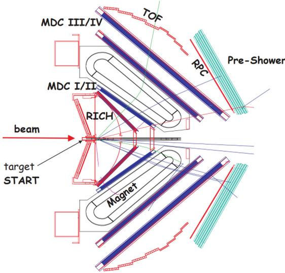
Fig. 1. Schematic expanded view of the HADES setup [18].
