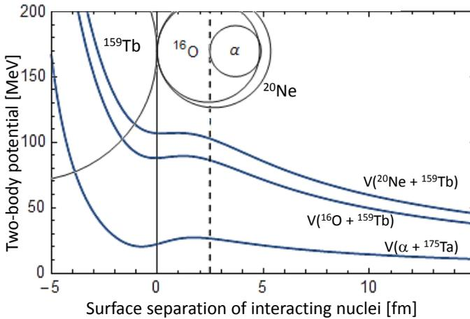
Fig. 3. Geometry of the projectile approaching the target, and the corresponding potentials ( $l_i = 55$ ,  $l_n = 44$ ,  $l_\alpha = 11$ ) for the entrance channel  ${}^{20}\text{Ne} + {}^{159}\text{Tb}$  and for the two fragments when considering the incomplete fusion reaction  ${}^{20}\text{Ne} + {}^{159}\text{Tb} \rightarrow \alpha + {}^{175}\text{Ta}$ .
