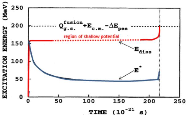
Fig. 4. Principle of the neutron clock: The time region indicated by the dashed line is adjusted to correspond to the number of neutrons emitted isotropically relative to the center-of-mass frame. Adapted from [14].
