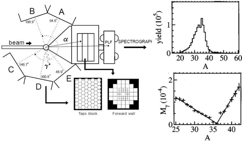
Fig. 2. The 5 TAPS blocks with  $\text{BaF}_2$  crystals detect energetic photons from nuclear bremsstrahlung. PLFs are detected with the GANIL spectrograph SPEG. In combination with the KVI Forward wall, it is possible to reconstruct the primary PLFs. The mass distribution is shown in the top panel. The probability, of the order of  $10^{-4}$  (!) to observe a high-energy photon together with a primary PLF is shown in the lower panel. Note the different mass scales on the horizontal axis.
