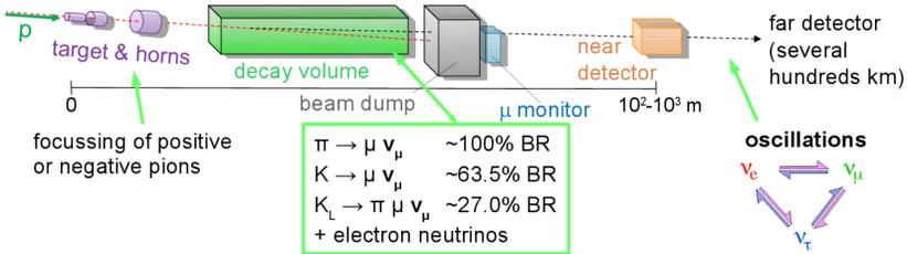
Fig. 1. Neutrino beam production. By focussing positive or negative pions, one can obtain a beam in neutrino or antineutrino mode.
