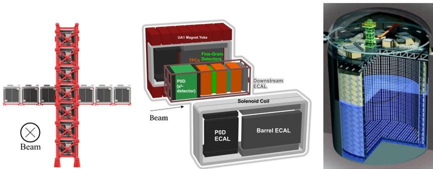
Fig. 3. Detectors relevant for T2K oscillation analysis (not to scale). Left: on-axis near detector INGRID. The nominal neutrino beam axis goes through the central part of INGRID, in the inward direction in this graphic. Middle: off-axis near detector ND280 (exploded view). Right: far detector Super-Kamiokande.
