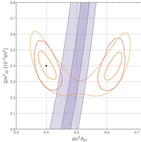
Fig. 2. (Colour on-line) Predicted 90% C.L. sensitivity for T2K after 7.8e21 POT (black/red) and NOvA (grey/orange) after 1.2e21 POT (grey/solid) and 6e21POT (grey/dashed), for the true values  $\sin^2 \theta_{23} = 0.4$ ,  $\Delta m_{32}^2 = 2.4 \times 10^{-3} \text{eV}^2$ . The regions allowed by CSD(3) are shown after the restricting  $\theta_{13}$  and  $\Delta m_{21}^2$  to their NuFIT  $1\sigma$  and  $3\sigma$  ranges.
