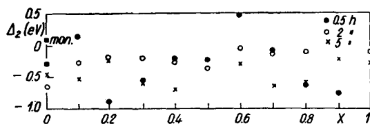
Fig. 6. Generation energy \Delta_2 of electric current carriers as a function of the composition of specimens sintered at 1470°K during 30 min, 2 hrs and 5 hrs, respectively, in the absence of magnetic ordering
